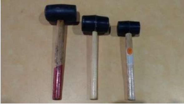
Three mallets of different sizes (large, medium, small) with wooden or metal handles.                                      | Maillets de différentes tailles<br>Total : 3             |
